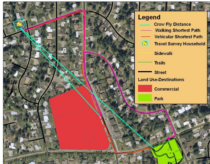
Figure 4 Process for Measuring Route Directness by Mode
